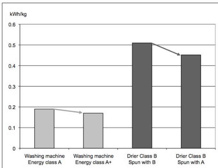
**Figure 1. Energy consumption and energy savings per kg of laundry according to higher efficiency classes for washing and spinning (with drier class B), related to the old EU energy label, calculated by Topten<sup>18</sup>.**
