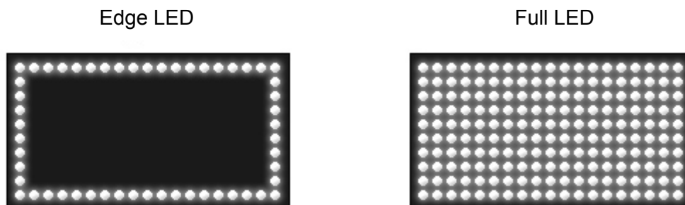
Figure 4: Two different types of LED-Backlighting: Edge LED resp. Full LED (Source: tvfacts.de, 2010)
