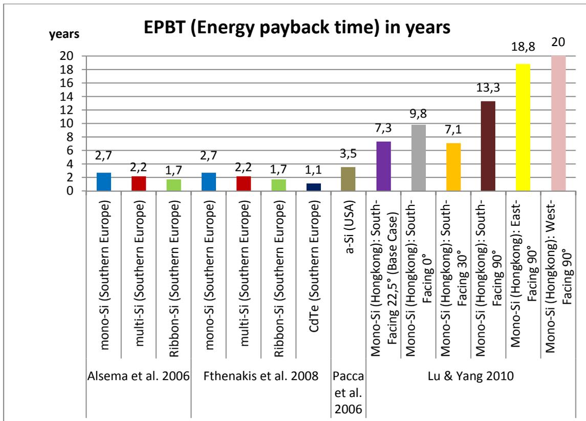
Figure 6: Compilation of EPBT calculation from different sources (author's own diagram based on Gröger et al. 2013) Pollutants – Cadmium (Cd). Note: mono-SI = sc-SI; multi-SI = mc-SI
