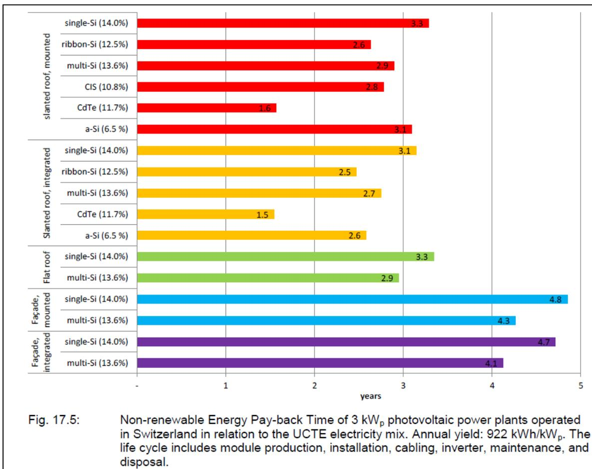
Figure 5: Comparative evaluation of PV systems with different module types in terms of their energy payback time (EPBT) (figure directly sourced from Jungbluth et al. 2012). Note: single-SI = sc-SI; multi-SI = mc-SI
