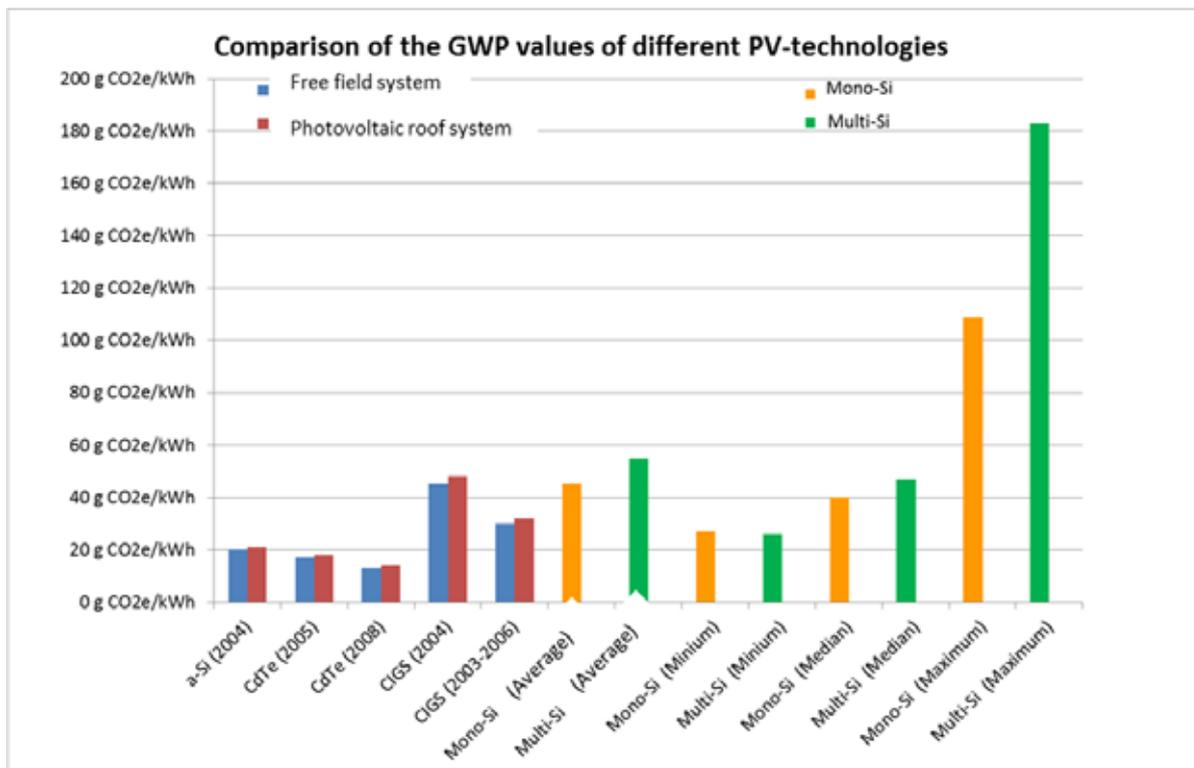
Figure 3: Comparison of harmonized GWP values of different PV modules (data from Hsu et al. 2012, H.C. Kim et al. 2012) Note: mono-Si = sc-Si; multi-Si = mc-Si
