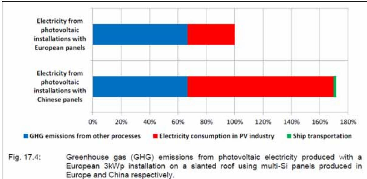
Figure 4: Greenhouse gas emissions from multi-Si modules installed on a slanted roof, based on the assumption that a European and a Chinese electricity mix, respectively, will be used for production (figure directly sourced from Jungbluth et al. 2012)
