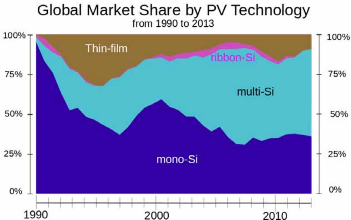
Figure 2 Global market-share by photovoltaic technology from 1990 to 2013, in terms of annual worldwide production. Technologies include as follows, crystalline silicon (c-Si) encompassing monocrystalline silicon (mono-Si), polysilicon (multi-Si) and ribbon silicon (ribbon-Si), as well as thin-film technology, including amorphous silicon, CdTe and CIGS. Source: Fraunhofer ISE, Report, current edition data from archived edition, July 28, 2014, page 18 via Wikipedia 2014
