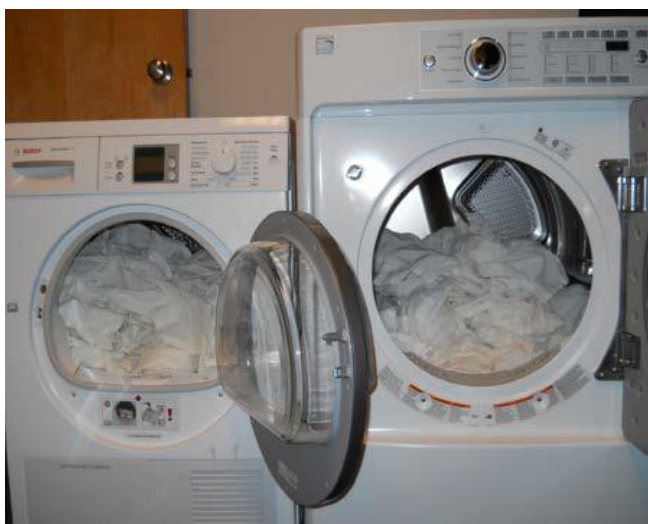
Figure 5: Drum size difference: European drier (left) and North American (right) drier [12].
