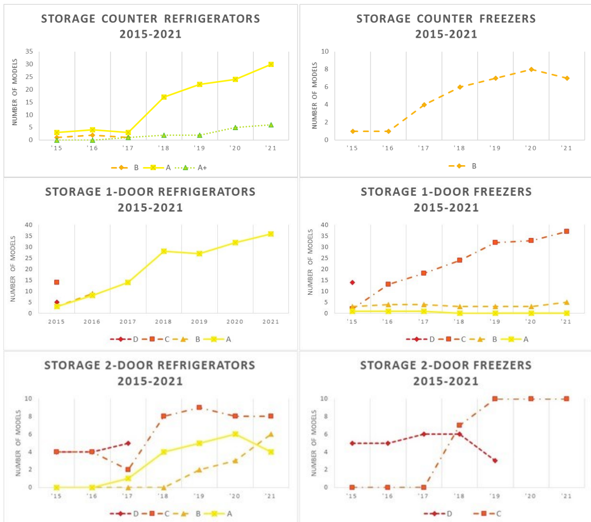
Figure 1: Market development of BAT models for professional refrigerated storage appliances from 2015-2021 by category. Data & Graph: Topten.eu
