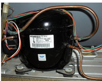
Figure 13: Fixed speed compressor (on/off)
