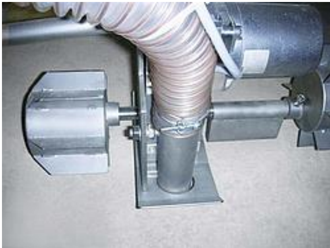
Picture 21: a mobile suction probe, called Mole
