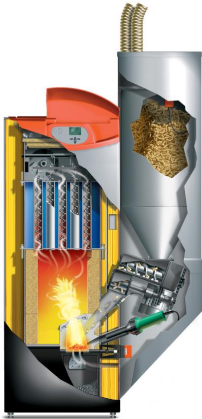
Picture 15: 3D-cut of a pellet boiler with a drop system
