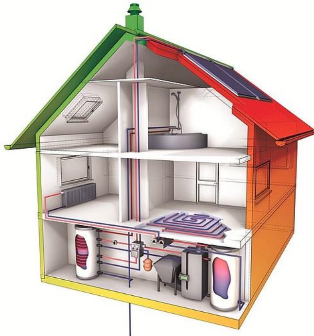
Picture 3: Functionality of heating systems with a pellet boiler, solar hot water generation
