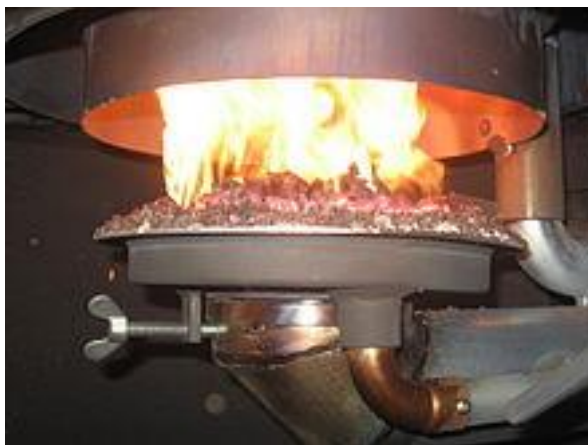
Picture 13: The retort firing system in detail (the pellets are pushed upwards)
