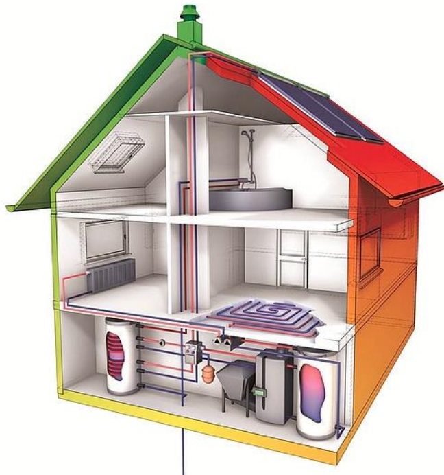
Picture 2: Functionality of heating systems with a pellet boiler, solar hot water generation
