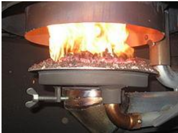
Picture 12: The retort firing system in detail (the pellets are pushed upwards)
