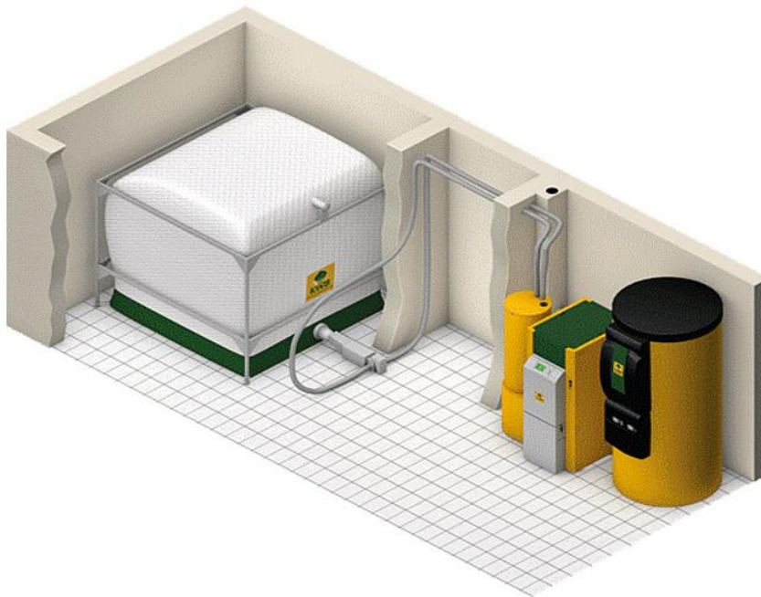
Picture 22: pneumatic suction from a big bag into the boiler
