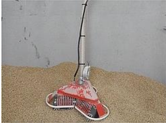
Picture 19: a mobile suction probe, called Mole
