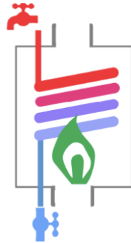
Figure 5: Schematic representation of a gas-fired instantaneous water heaters
