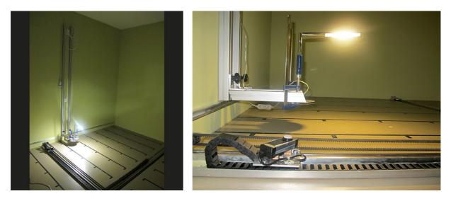
Figure 4: Standardized room for measuring household luminaires at the University of Applied Sciences HTW Chur. A robot measures the illuminance at 100 points on the ground surface. Further parameters are energy consumption (use and standby), color rendering index CRI, color temperature, direct glare and dimming (leading edge / trailing edge).
