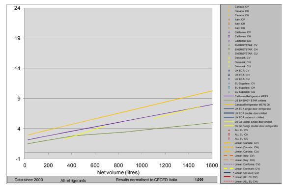
Figure 9. MEPS for chilled cabinets (note: ENERGY STAR line being checked, potential error)
