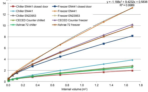
Figure 7. Graph of energy consumption per 24 hours against cabinet volume for upright cabinets according to different test methodologies, showing results from the mathematical model.
