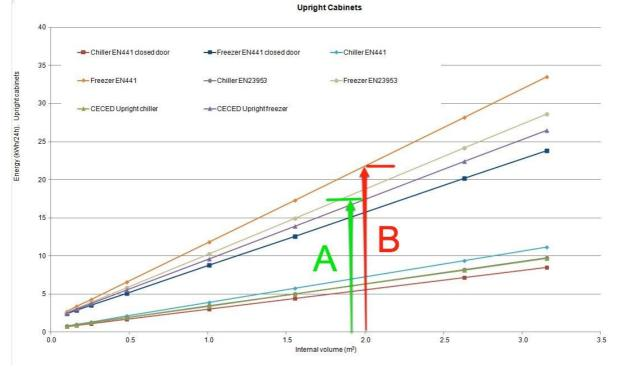
As an example calculation step: in Figure 8 the energy consumed by a 2 m<sup>3</sup> upright freezer cabinet tested according to EN441 is around 22 kWh (dimension B) per 24 hours; and for the same cabinet under CECED Italia 17.5 kWh (dimension A). So a test result under EN441 should be adjusted by the ratio:
