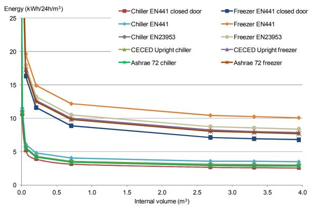
Figure 4. Predicted energy consumption per cubic metre of net volume for an horizontal cabinet according to the different test regimes.
