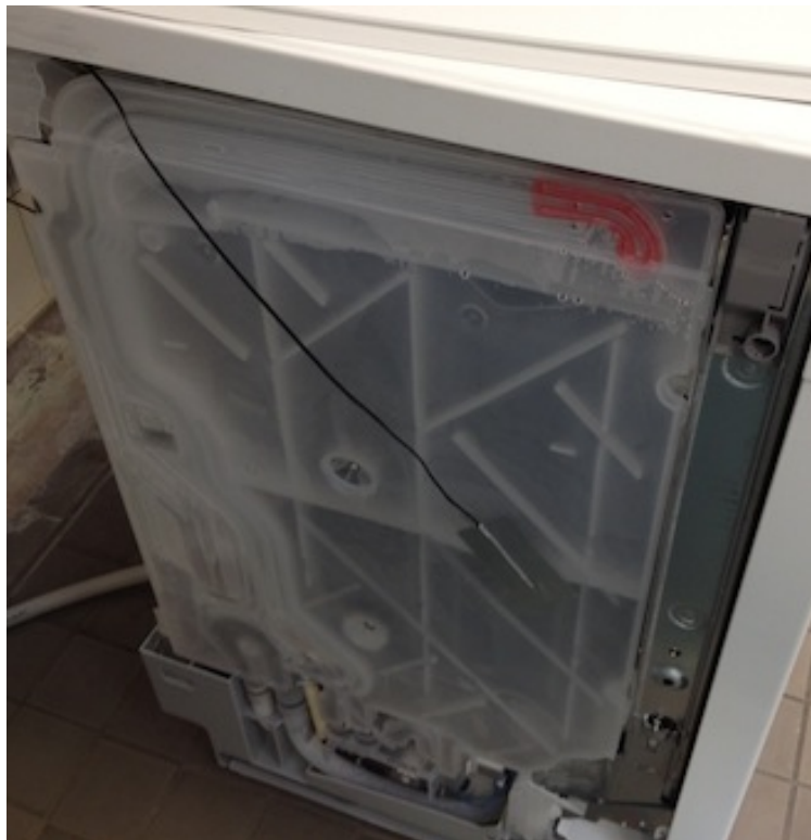
Figure 32: Water tank attached to the side of the Bosch dishwasher model.
