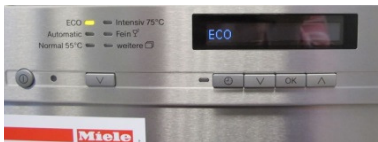
Figure 31: Programme selection panel of the Miele G-6300 SCU. Image source: VDE
