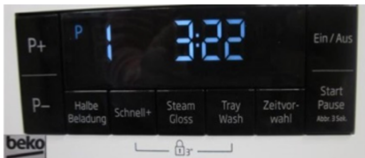
Figure 28: Programme selection panel of the Beko DFN26220S. Image source: VDE
